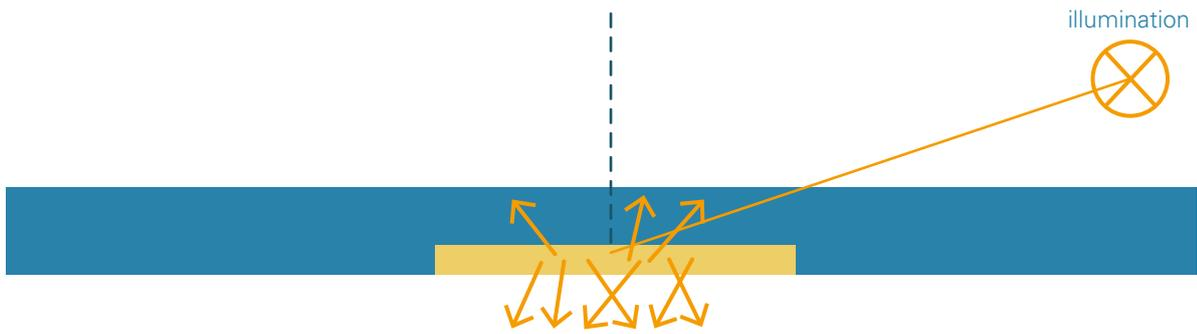
Fiducial marking structure etched and filled with pigment particles assuring light scattering
