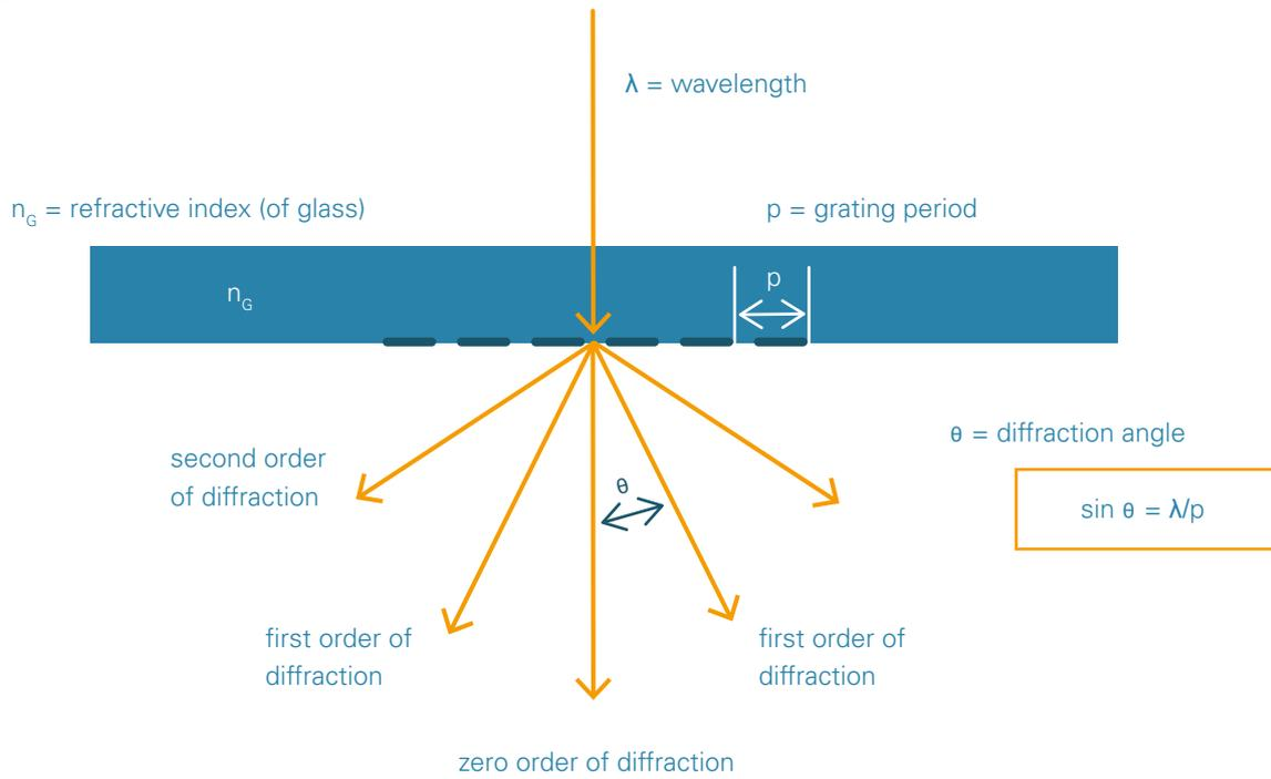
**Figure 2 |** Use of the first diffraction order
