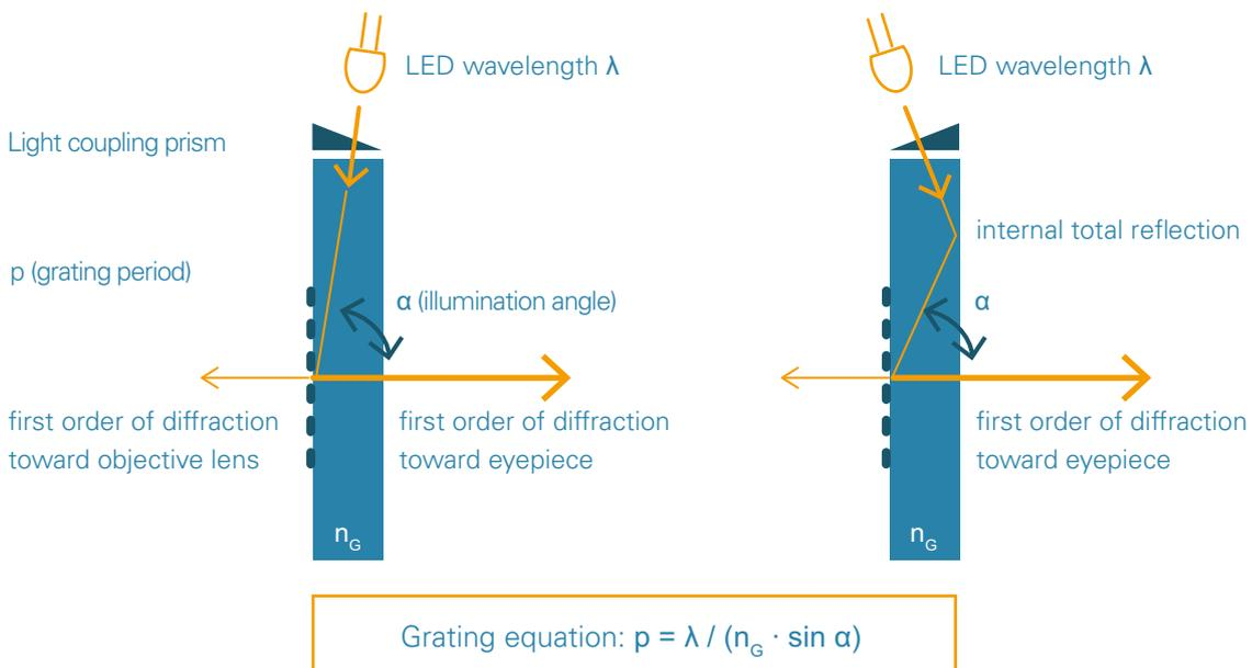
**For an ideal use of diffraction gratings the following parameters need to be considered:**
