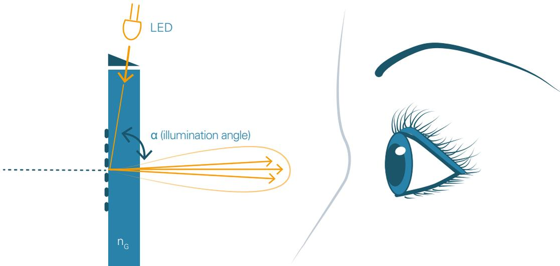
**Figure 4 |** Orientation of the light source
