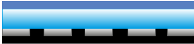
Combined high-/low-reflection pattern in the same focal plane in combination with a transparent anti-reflex optical coating for optimum transmission
