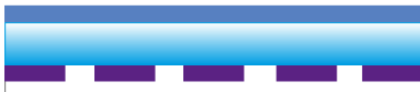
Combined low-reflection dark pattern/low-reflection white pattern in the same focal plane in combination with a transparent anti-reflex optical coating for optimum transmission
