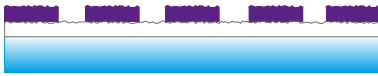
Low-reflection dark pattern/structure on no-reflection white diffusive surface (IMT DS) for specular-free reflection for machine vision applications
