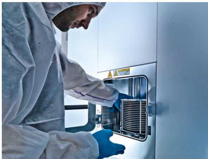
3 Automated fabrication and handling systems – here the load-lock of the sputtering system – mean that many of those manufacturing aspects so critical to the semiconductor industry – cleanliness, high volume and high yield in combination with cost-effective manufacture, singulation capability et cetera – are also common to IMT's workflow. (Source: Evatec)
